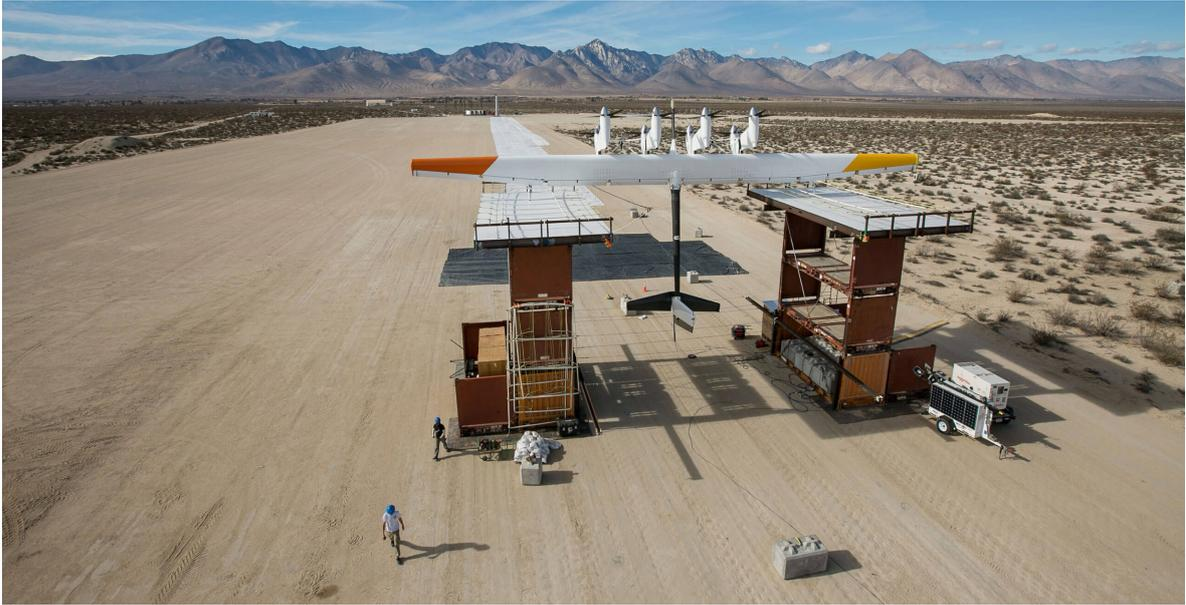
Figure 2.6: Makani 600 KW prototype [17].
