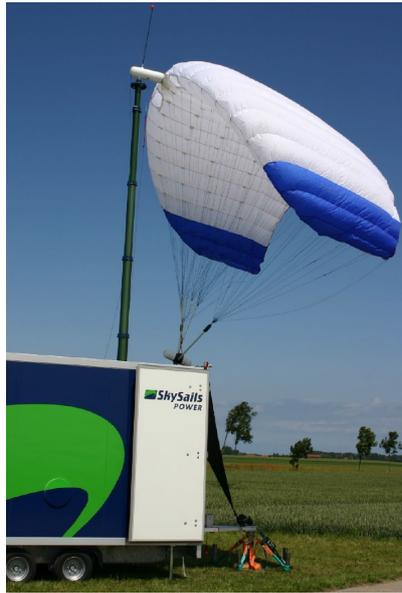
Figure 2.9: 55 KW Skysail Demonstrator [28].
