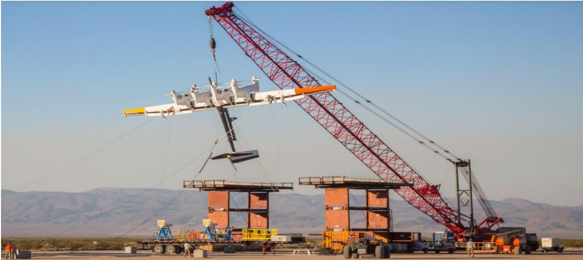
**Figure 2.14:** (Google-X) Makani Power 600 KW M600 Prototype[17].
