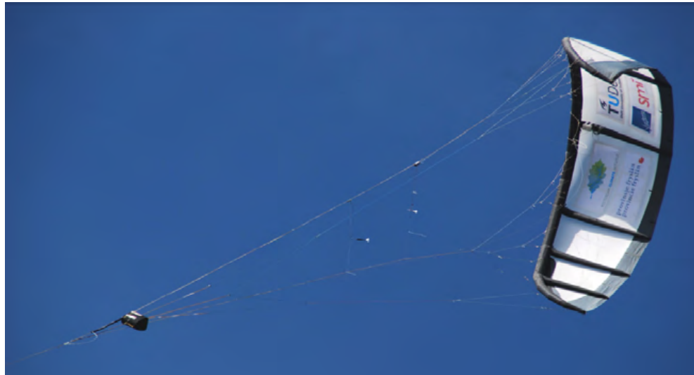
Figure 2.10: 20 KW Kitepower demonstrator [29].
