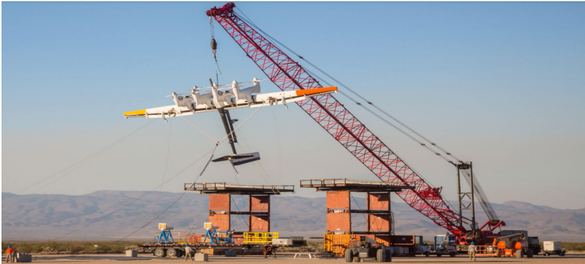
Figure 2.14: (Google-X) Makani Power 600 KW M600 Prototype[17].
