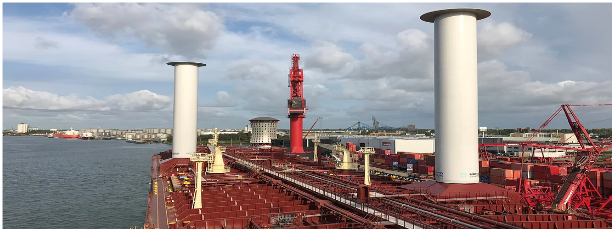
Figure 3.10: Maserk tanker with installed rotor propulsion system by Norsepower [89].
