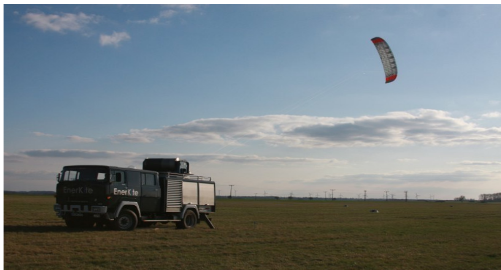
Figure 2.11: Enerkite 30 KW demonstrator [24].
