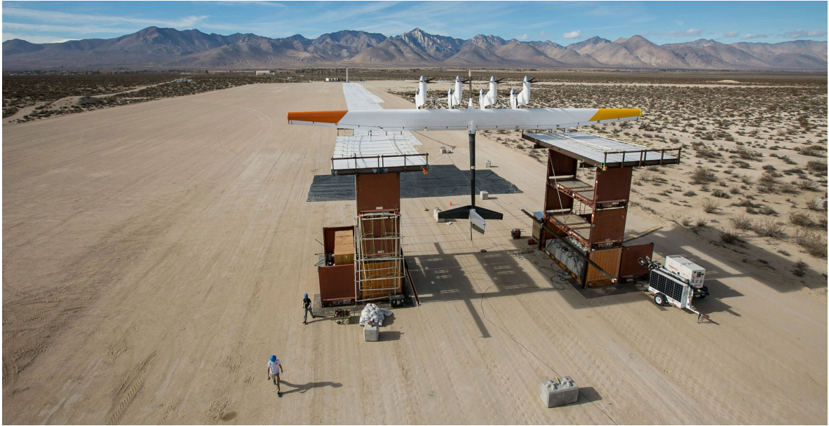
Figure 2.6: Makani 600 KW prototype [17].
