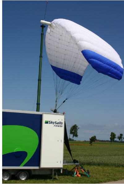
Figure 2.9: 55 KW Skysail Demonstrator [28].
