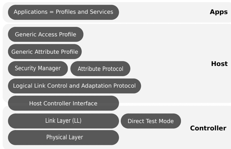
Figure 2.1: BLE Protocol Stack
