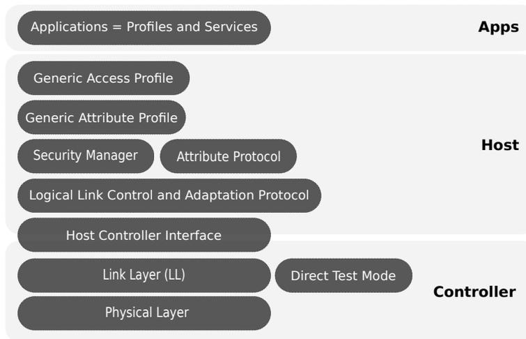
Figure 2.1: BLE Protocol Stack
