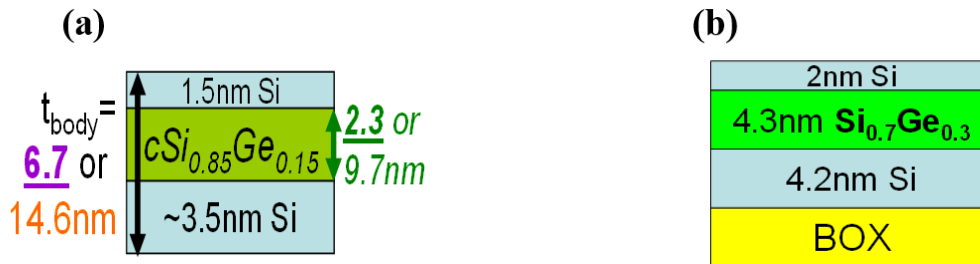
Figure 2.22. Schematics of ultra-thin body thickness (a) to study the impact of body thickness reduction and (b) to characterize the impact of the annealing temperature [61].
