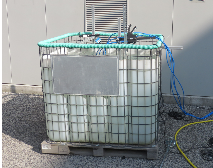
FIGURE 3.13 – Cuve de 1 \text{ m}^3 ( 1 \times 1 \times 1 \text{ m} ) utilisée pour les expériences à Irstea Lyon 1 m 3 water tank (1 × 1 × 1 m) used à Irstea Lyon for the experiments. The choice of this tank was made mainly because of its availability.
