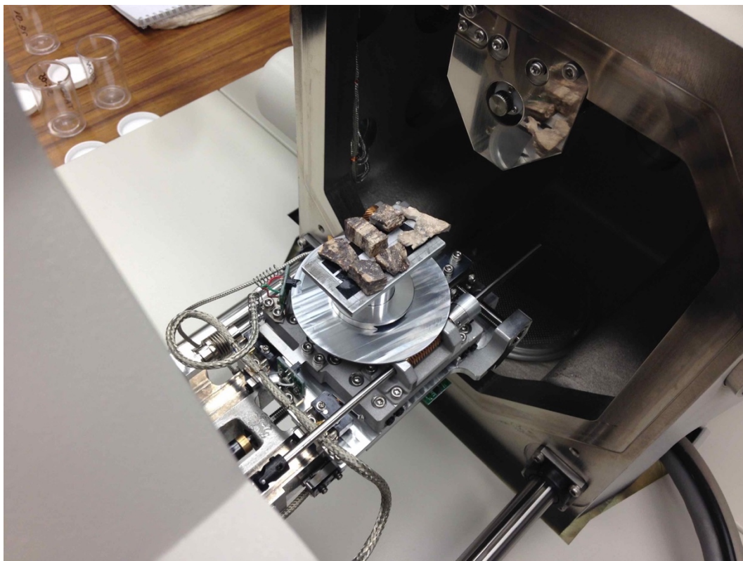
Figure 56. Initial attempt at a single EDS run of all six samples.
