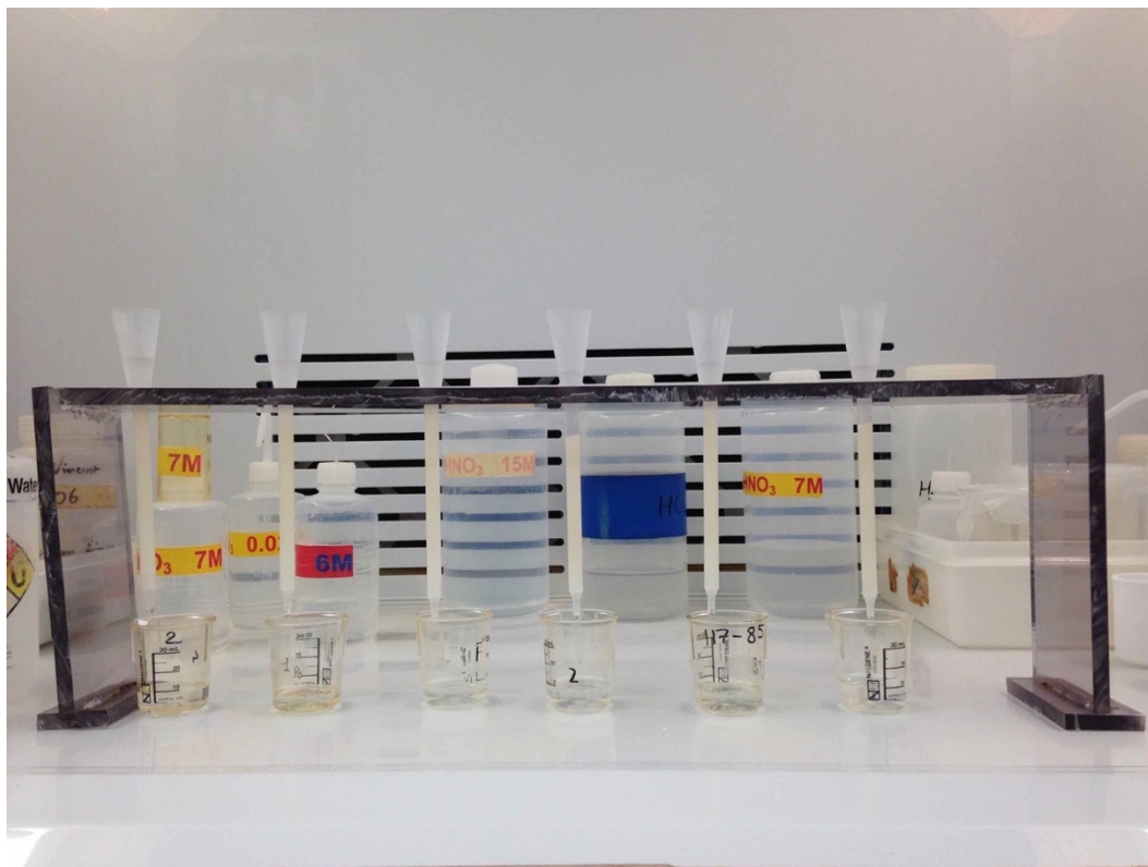
Figure 59. The first column array undergoing resin conditioning.
