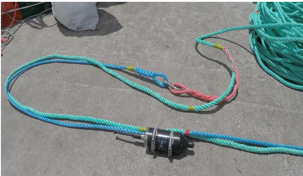
Figure 3-2 – Picture of the attachment of the SoundTrap on the downline (green rope). The SoundTrap is set permanently on a small rope (the blue one) to facilitate the deployment on the downline.
