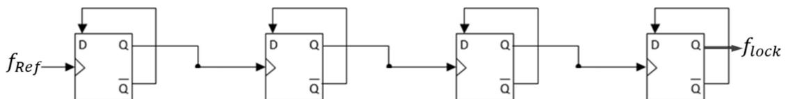
Figure 3.44: Frequency divider circuit.
