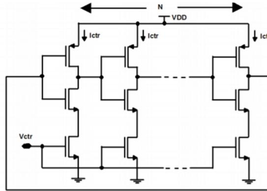
Figure 1. 23: Ring oscillator based VCO (Nebhen et al. 2012).
