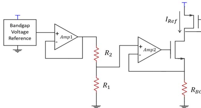
Figure 3.27: Architecture of the biasing block core.
