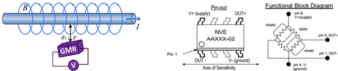
GMR current sensor (Ouyang et al. 2012)      GMR sensor from NVE (“NVE AA and AB-Series Analog Sensors” n.d.)
