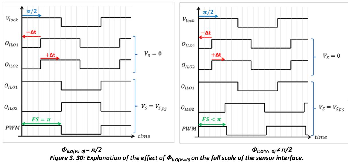
Figure 3.30: Explanation of the effect of  $\Phi_{ILO(V_S=0)}$  on the full scale of the sensor interface.
