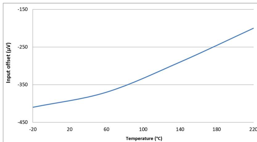
Figure 4.13: Measured input offset for different temperatures.
