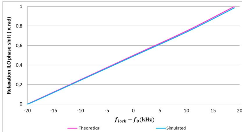
Figure 3.7: Phase shift of Relaxation Injection Locked Oscillator.
