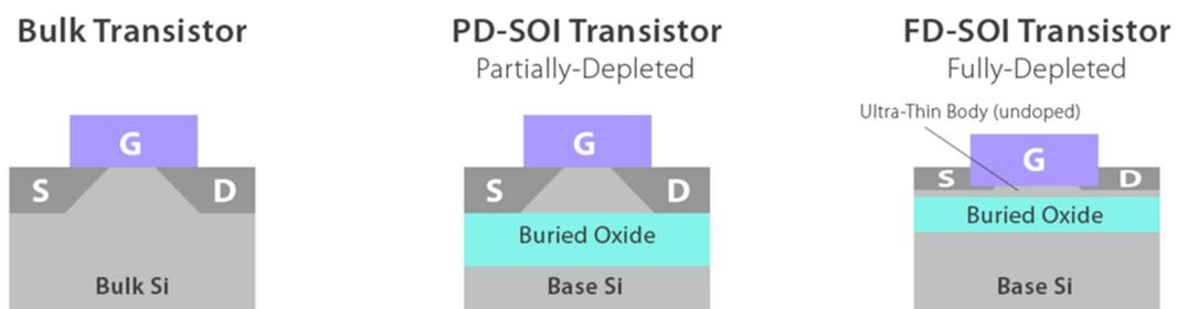
Figure 1.3: Structure of Bulk transistor, PD-SOI transistor and FD-SOI transistor (Olejarcz et al. 2012) .
