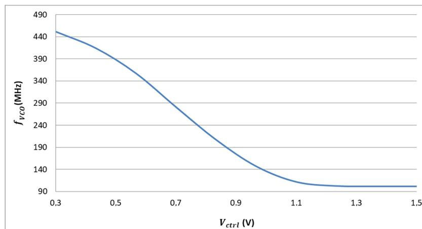
Figure 3.40: Characteristic function of the VCO at 27°C.
