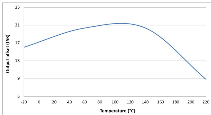
Figure 4.14: Measured output offset for different temperatures.
