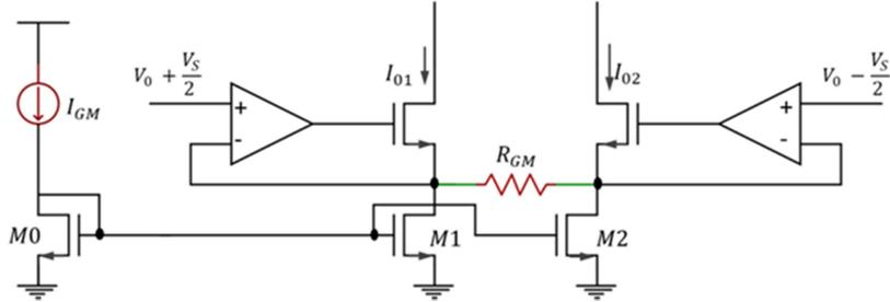
Figure 4.17: Transconductance amplifier.
