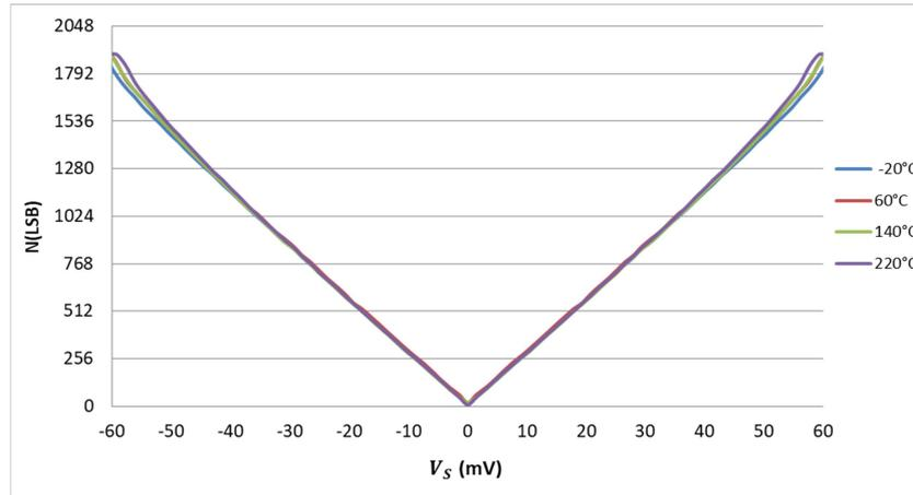
Figure 4.6: Experimental transfer function of the sensor interface [ $-20^{\circ}\text{C}$ ;  $220^{\circ}\text{C}$ ].
