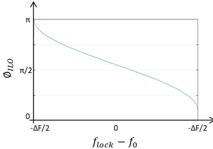
Figure 2.5: Phase shift of harmonic Injection Locked Oscillators.
