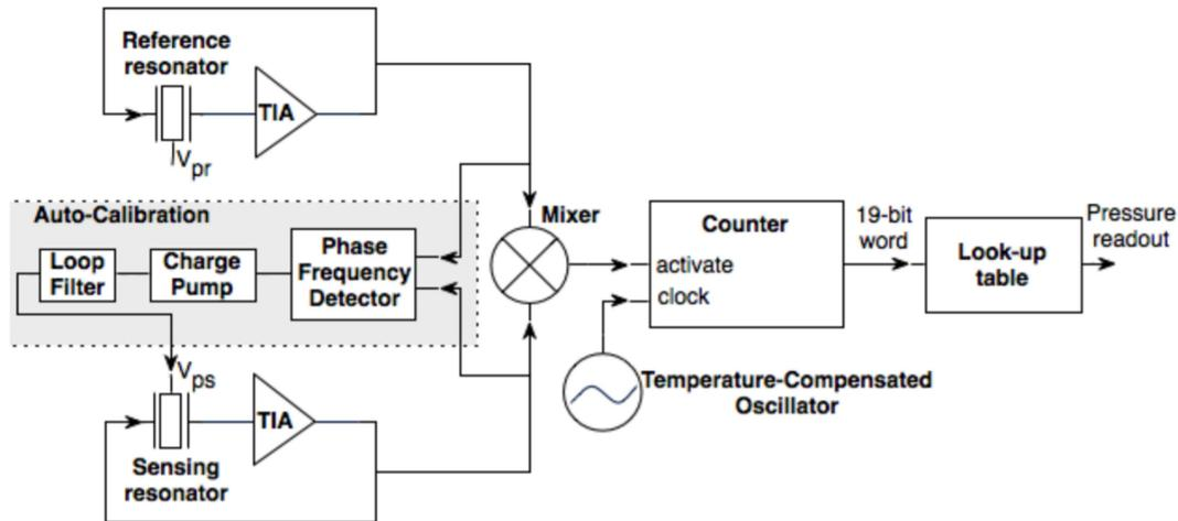
Figure 1. 21: Differential sensor readout circuit (Taghvaei et al. 2010) .
