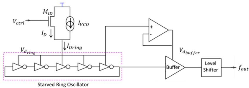
Figure 3.39: Topology of the voltage controlled oscillator.
