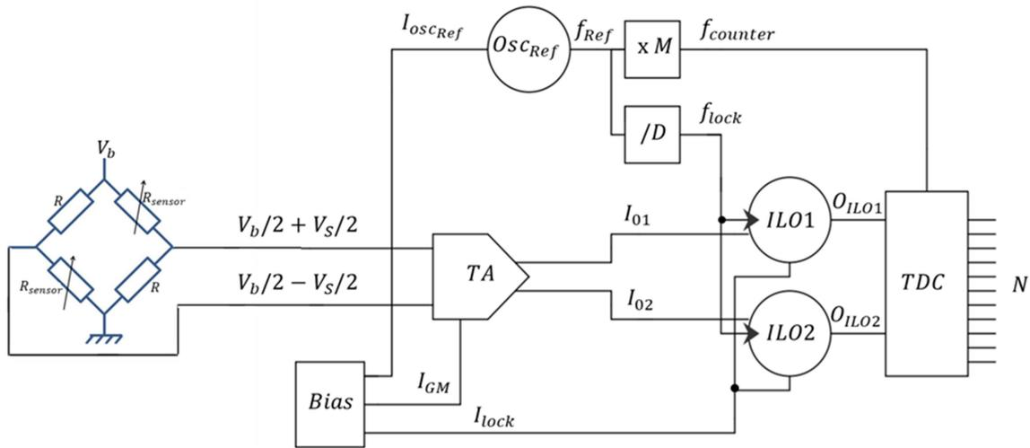
Figure 3.8: Sensor interface circuit based on Relaxation ILOs.
