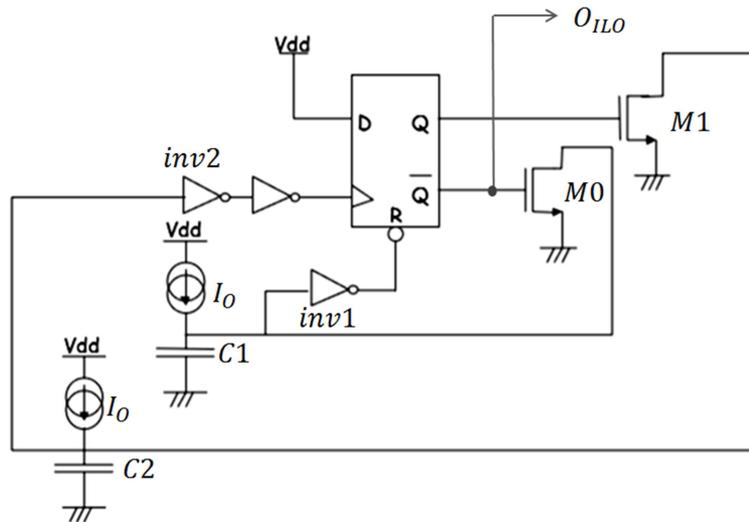
Figure 3.2: Schematic of relaxation free running oscillator.
