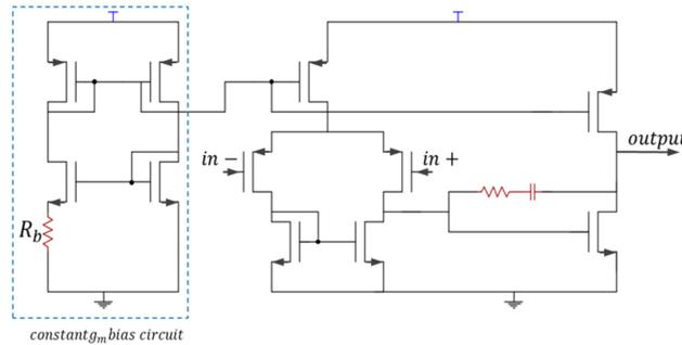
Figure 3.13: Architecture of the operational amplifier (OPA) using the constant  $g_m$  bias circuit.
