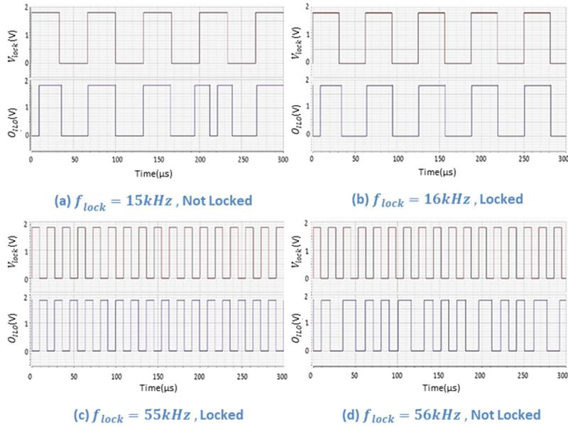
Figure 3. 6: Simulation of the Relaxation Injection Locked Oscillator for different locking frequencies.
