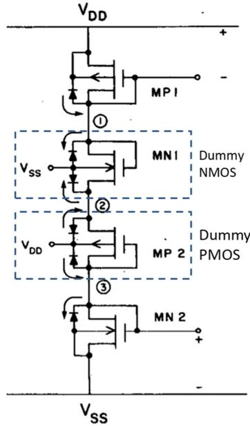
Figure 1. 17: Leakage current matching technique (Shoucair 1986) .
