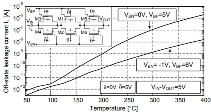
Figure 1. 19: OFF\_state leakage current reduction using RBB in an analog switch ( $V_{BN}$  and  $V_{BP}$  are respectively the reverse bias voltage of the NMOS and PMOS transistors) (A. Schmidt, Kappert, and Kokozinski 2013).
