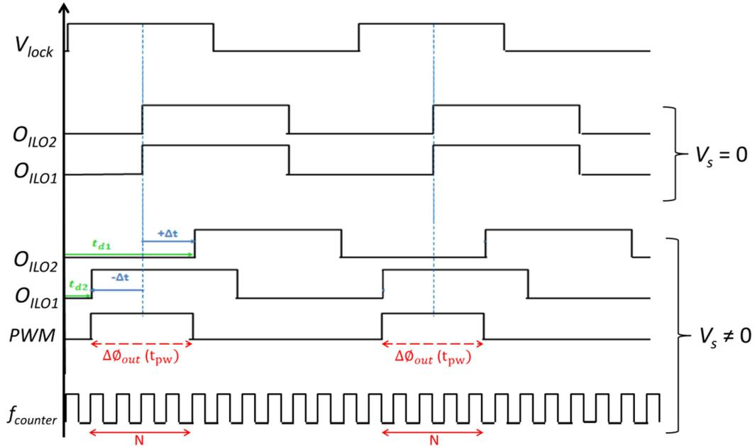
Figure 2.10: Timing diagram of the sensor interface architecture.
