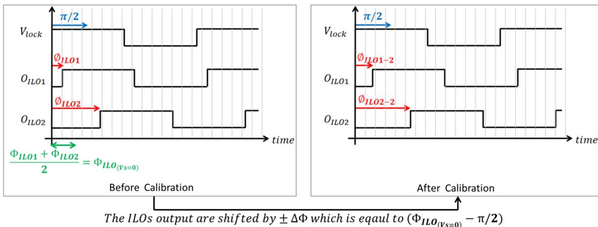
Figure 5. 1: Principle of the auto-calibration loop.
