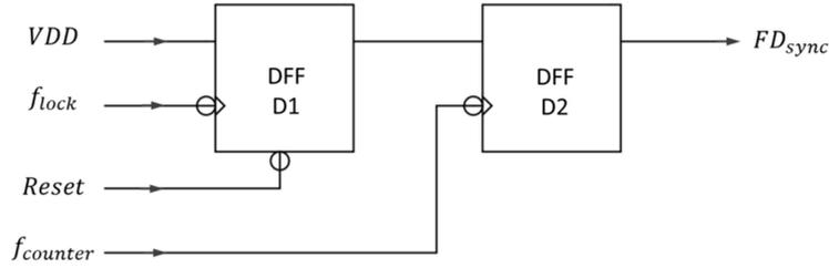
Figure 3.32: Detector circuit of the falling edge of  $V_{lock}$ .
