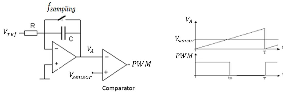
Figure 1. 24: Pulse Width Modulation technique (PWM).
