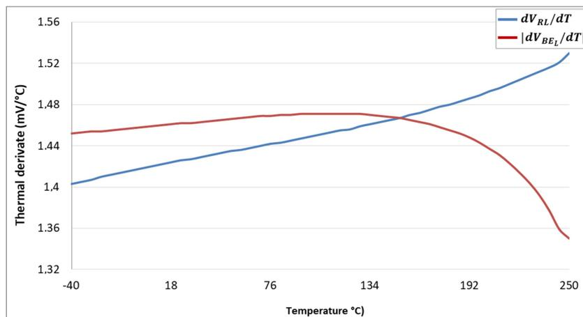
Figure 3.24: temperature sensitivity of  $V_{BE_L}$  and  $V_{RL}$ .
