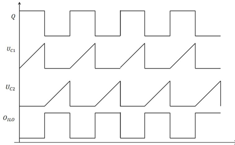
Figure 3.3: Timing diagram of the free running oscillator.
