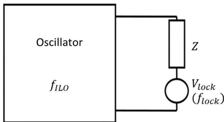
Figure 2.3: Injection Locked Oscillators representation (Franck Badets 2000).
