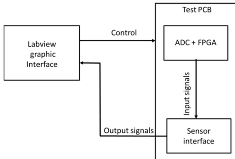
Figure 4.3: Principle of the measurement test bench.
