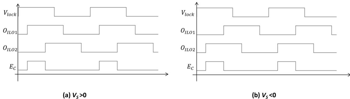
Figure 3.31: Chronograms of the counting enable signal  $E_C$ .
