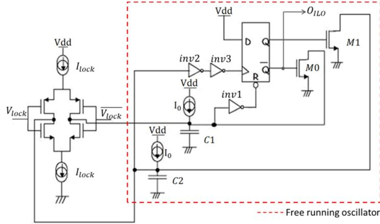
Figure 3. 4: Schematic of the Relaxation Injection Locked Oscillator.
