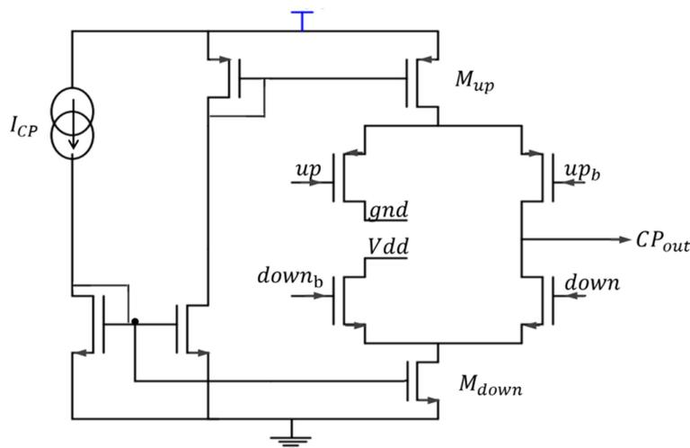
Figure 3.37: Charge pump circuit with current steering switchers.
