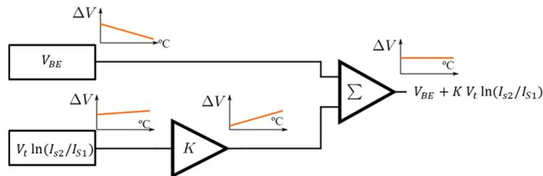
Figure 3.20: Principle of the bandgap voltage reference.
