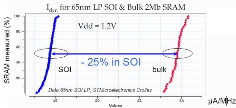
Figure 1. 6: Dynamic power reduction in SOI transistors (Martineau 2008).
