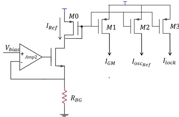
Figure 3.28: Generation of  $I_{GM}$ ,  $I_{oscRef}$  and  $I_{lock}$ .
