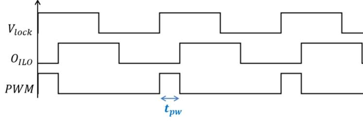
Figure 2.7: Representation of the output PWM signal.
