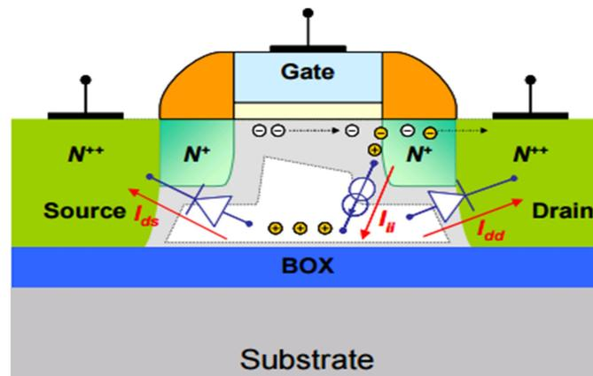
Figure 1. 14: Impact by ionization effect in PD-SOI (Martineau 2008) .
