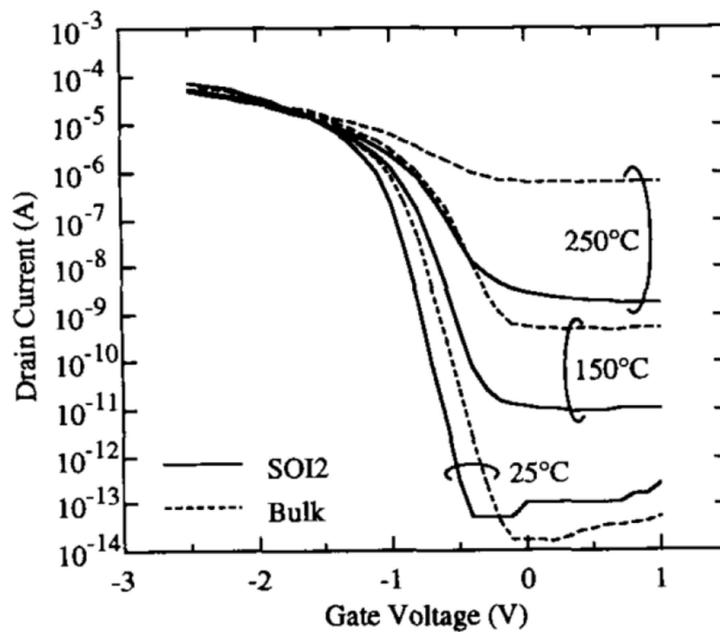
Figure 1. 10: Drain current as a function of  $V_{gs}$  of SOI and Bulk transistors (Arbess 2012) .
