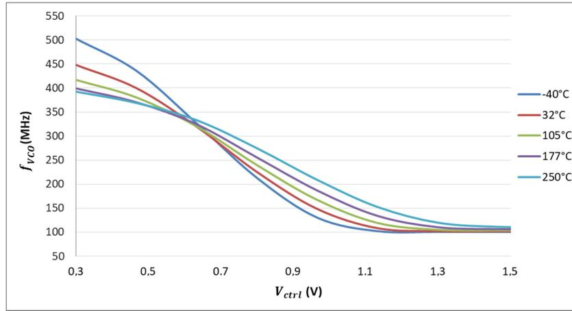
Figure 3.41: VCO characteristic function for different temperatures.
