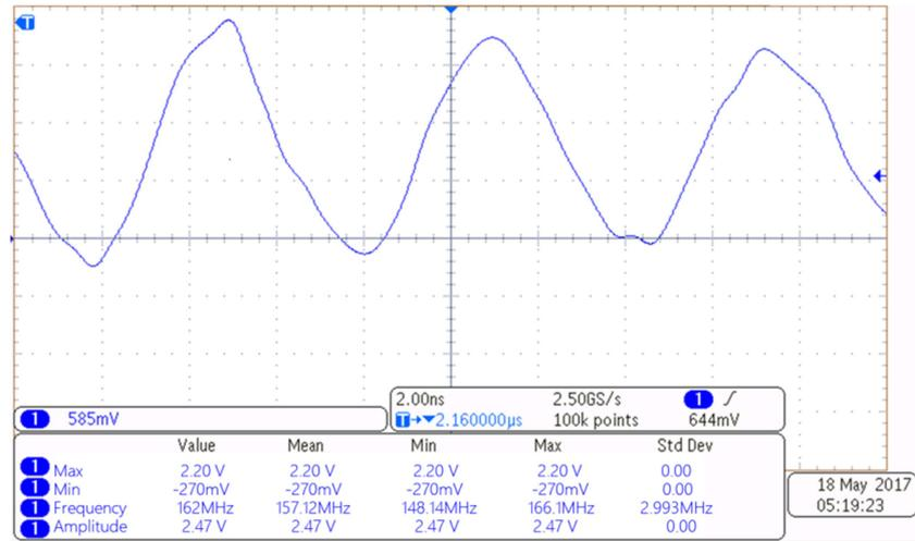
Figure 4.10: Visualisation of the counter clock signal.
