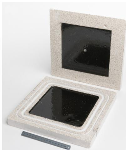
FIGURE 3.4: Mold design for experimental tests in the microwave oven
