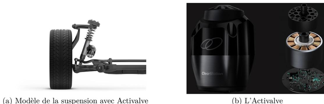
FIGURE 2.6 – La suspension active ClearMotion
