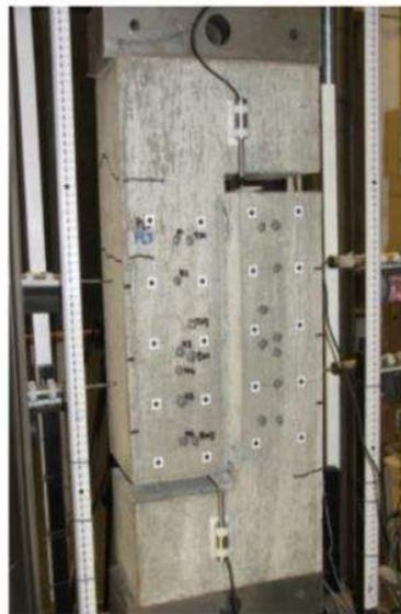
**Figure 1.3 :** Essai Push-off.
