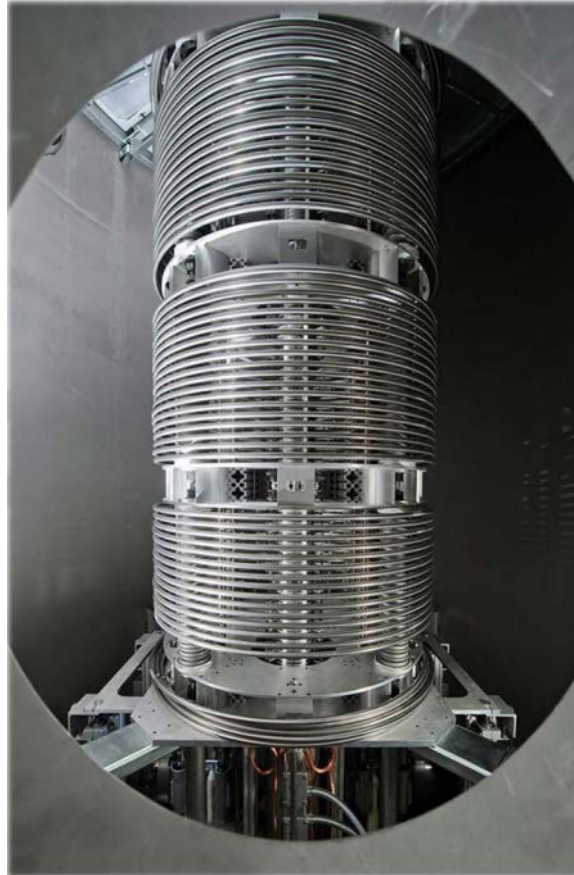
FIGURE 3.3: View of the 3 acceleration sections at the bottom of the accelerator inside the Sta. Ana accelerator tank.
