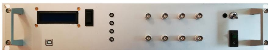
**Figure B.15:** Front panel of the security system. USB: programming port, BNC: Inputs for temperature sensors or interlocks, Button (left): menu, Button (lower right): On/off switch for the monitoring electronics, Flip switch (upper right): Day/night mode.
