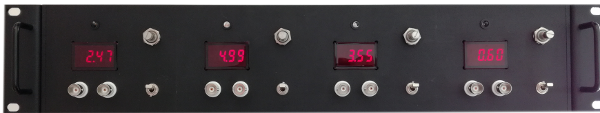
Figure B.18.: Front panel. Switch: remote control (LED on) or local override mode (LED off). BNC connectors: Analog and digital modulation channels of the RF drivers (blocked in override mode). Potentiometer: analog tuning voltage in override mode, displayed on the LCD panels.
