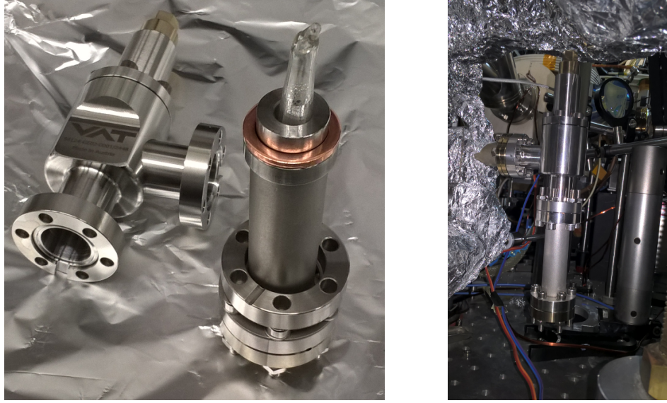
Figure B.19.: New Potassium reservoir. Left: custom stainless steel mount holding the ampule in place. The height ensures that the angle-valve can be used to crack open the ampule under vacuum. Right: reservoir after installation and additional bake-outs.
