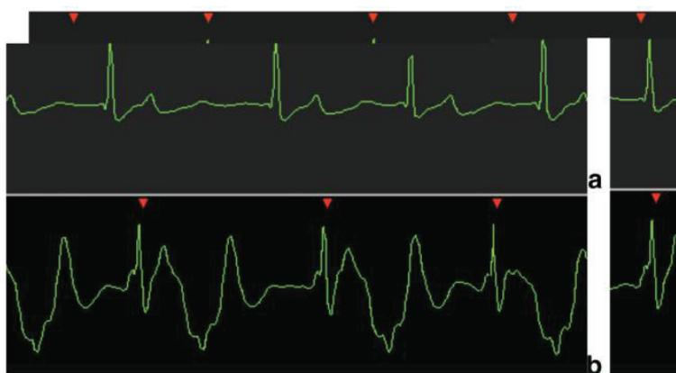
FIG. 2. **a,b:** Vector cardiogram traces of the aV<sub>f</sub> channel acquired (a) outside (approximately 0.5T) and (b) inside the 7T whole body magnet. The red arrows show the accuracy of the gating despite the severe magneto-hydrodynamic effect.
