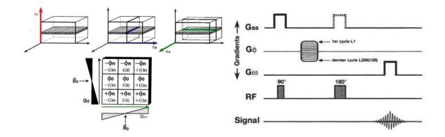
Figure 18: MRI spatial encoding. First is the selective slice excitation with a gradient across the slice **Gss**. Then is the line encoding with a phase-gradient  $G\varphi$ . Finally is the frequency encoding gradient  $G\omega$  during the readout of the echo that differentiate voxels along each line. Corresponding time diagram for a spin-echo MRI experiment is illustrated on the right panel (Kastler et al. 2006).
