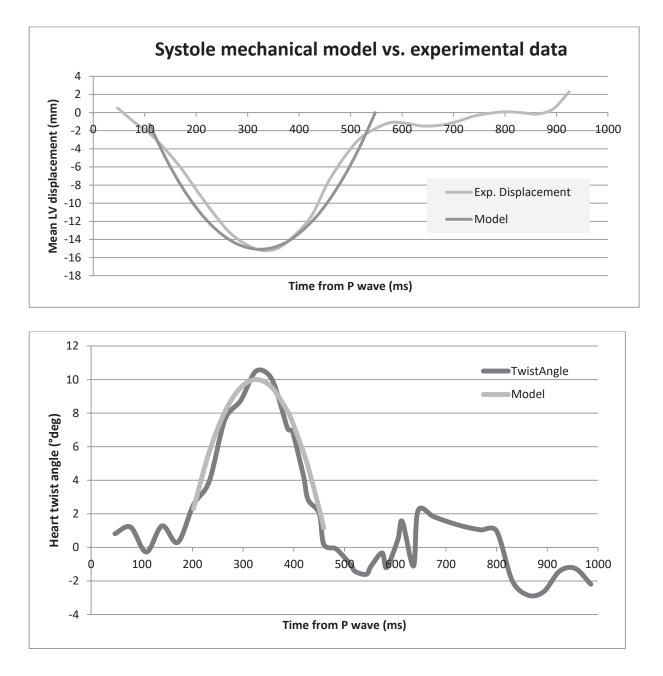
Figure 37: **TOP**: Simple mode for systole contraction fitted on experimental data (DENSE) from a volunteer;
