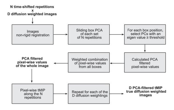
Figure 57: Block diagram of PCATMIP processing flow. Blocks represent processing steps and outputs are shown in bold. Transferred data is symbolized by arrows connecting blocks.
