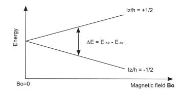
The splitting occurs because of the interaction of the magnetic moment  $\mu$  of the atom with the magnetic field **B** slightly shifts the energy of the atomic levels by an amount:
