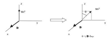
Figure 12: Rotation of macroscopic magnetization subject to a local radio-frequency variable electromagnetic field **B**<sub>1</sub>.
