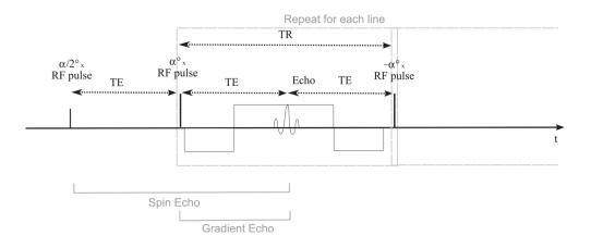
Figure 16: Schematic construction of a balanced-Steady State Free Precession (b-SSFP) MR sequence. The combination of a spin echo and a gradient echo creates a steady state after the second RF pulse  $(+\alpha^{\circ}_{x})$  that can be maintained with repeated RF pulses.
