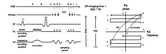
*Figure 20: Time-diagram of an Echo Planar Imaging (EPI)MRI spin-echo sequence. Corresponding lines letters are reported on the read k-space on the right panel(DeLaPaz 1994).*
