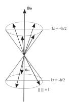
It is possible to show the rotation is limited to a cone, with a given cone angle  $\theta_m \approx 54.74^\circ$ .
