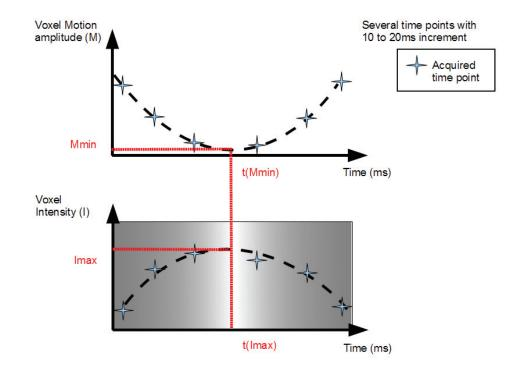
Figure 45: Time-Maximum Intensity projection (TMIP) principle to access motion-less diffusion-weighted signal intensity with trigger-shifted acquisitions
