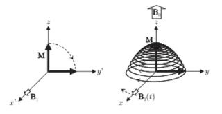
*Figure 13: Excitation (left) and relaxation (Right) of the macroscopic magnetization. The relaxation occurs in a spiral trajectory that rotates (=nutation) around the intense static field Bo.*
