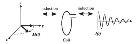
Figure 14: Basis of NMR excitation-reception. Excitation: an alternative current in the coil generates a variable magnetic field on the spin lattice. Reception: the magnetization generates a variable flux that induces electrical currents in the coil.
