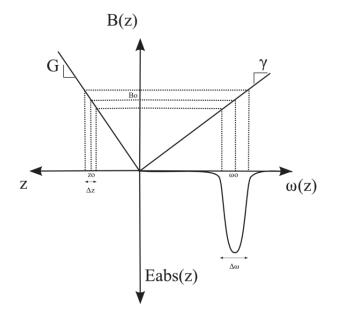
Figure 17: MRI slice selection principle. A magnetic gradient G creates a linear relationship between the magnetic field B and the spins location along the axis z: B(z). Thus spins resonance frequency depends on z according to the Larmor equation. Finally only the spins whose frequency is within range of excitation pulse frequency are excited: only a slice along axis z is excited.
