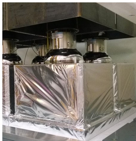
(e) Encapsulation of eight optical modules into the shielding.
