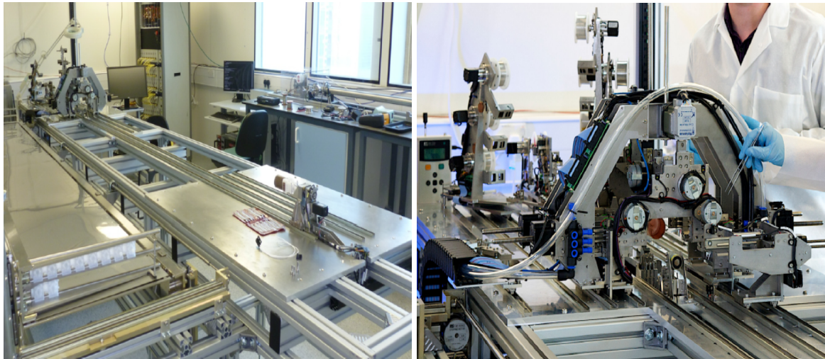
Figure 2.5: Photos of robot developed for the preparation of the tracker cells.
