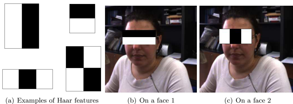
Figure 3.1: VJ face detection: Haar features applied on a facial image
