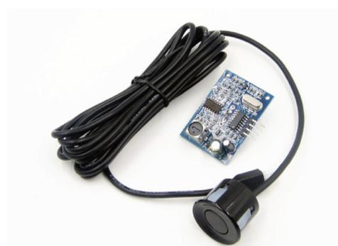
(a) Ultrasonic sensor and its electrical circuit board.
