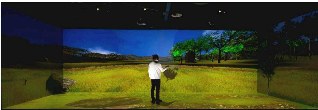
Figure 3.4 – Immersia is one of the largest VR research platforms in the world. It is composed of 4 large screens on which images are projected for a total volume of approximately  $90m^3$ . The 3D rendering is achieved by using active stereoscopic method associated with shutter glasses. 16 infrared cameras track the moving objects on the platform.
