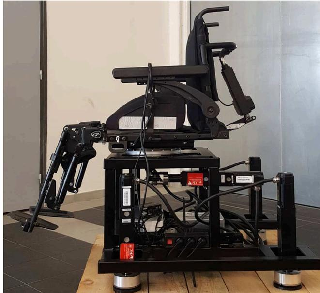
Figure 3.18 – Mechanical platform for enhanced virtual experience.
