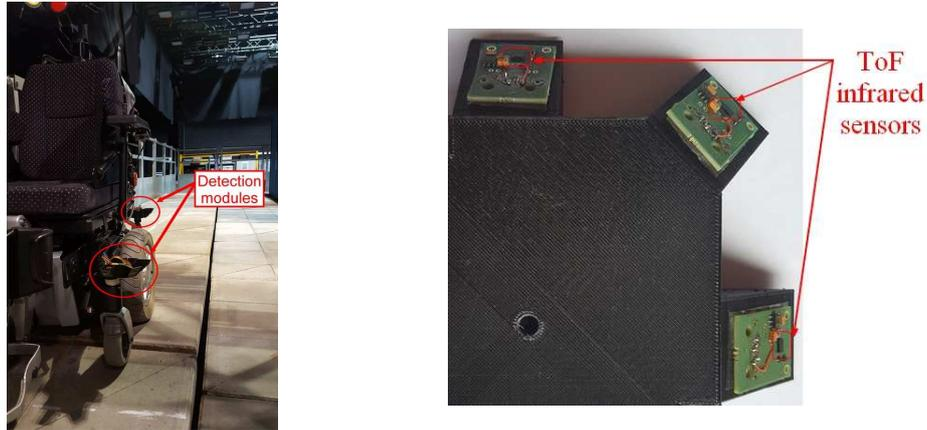
Figure 5.7 – (a) Power wheelchair equipped with detection module prototypes. (b) Detection module prototype (bottom view). Each detection module is composed of 3 ToF sensor boards inclined at 45 degrees to the vertical.
