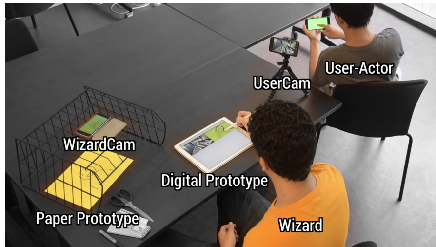
Figure 5.1: An overview of the MONTAGE video prototyping system. Here, two designers, a wizard and a user-actor, collaborate side-by-side. The UserCam captures the user-actor enacting user inputs in the actual context, i.e. using his phone at the office. The WizardCam captures the paper prototype and the Canvas captures the wizard's digital sketches.
