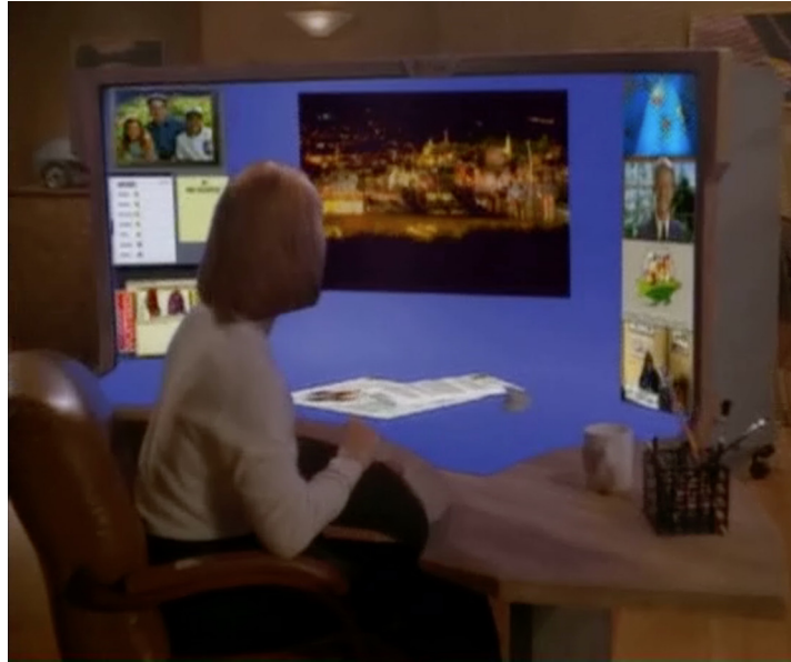
Figure 3.8: The prototype of an interactive curved desktop display. Placing objects on the flat area allows the system to scan the contact area, e.g., to scan a document. The workstation can be controlled with a mouse or via voice commands. From "The Starfire" by Sun Microsystem Inc.
