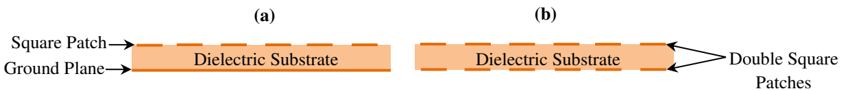
Figure 5. 11. Illustrations (Cross Section Views) of a grounded square patch panel implementing classical SIM (a) and double square patches panel implementing Generalized SIM with |\Gamma_G| = 1 (b).
