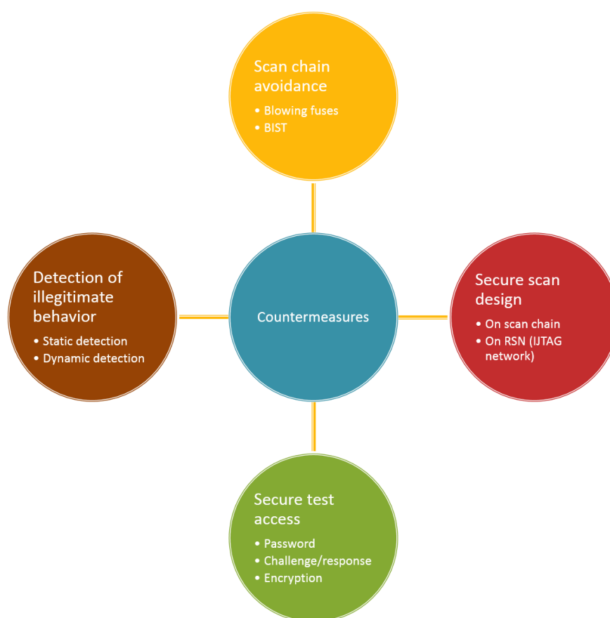
Figure 18: Classification of the countermeasures against the attacks using the test interfaces.
