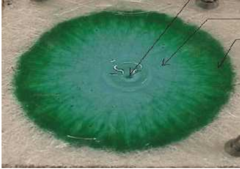
Figure 10: Colorant distribution at the end of the "two-color" central injection experiment in a single-scale porous material ([56])
