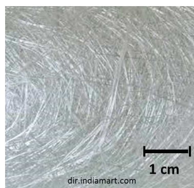
Figure 2: Example of a chopped fiber random mat
