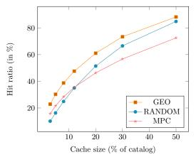
Figure 4.7: Hit ratio achieved for different content placements with user association maximizeing throughput under OPT- h and 1-freq.
