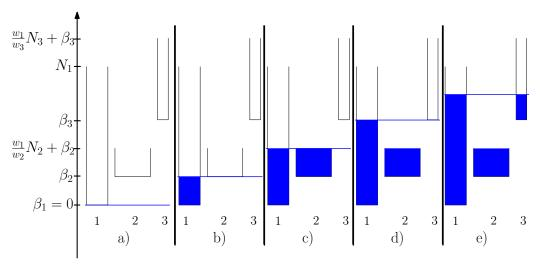
Figure 4.3: Illustration of the Bucket-filling algorithm.
