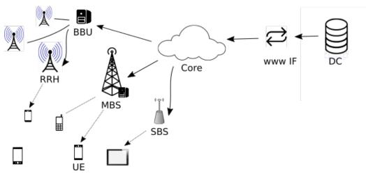
Figure 1.1: Content delivery in a wireless network.
