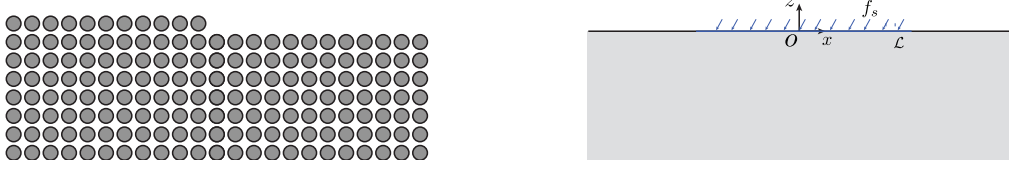
Figure 7.3: Representation in a continuum picture of the effect of a step on the bulk through a surface distribution of forces \mathbf{f}^s(x)
