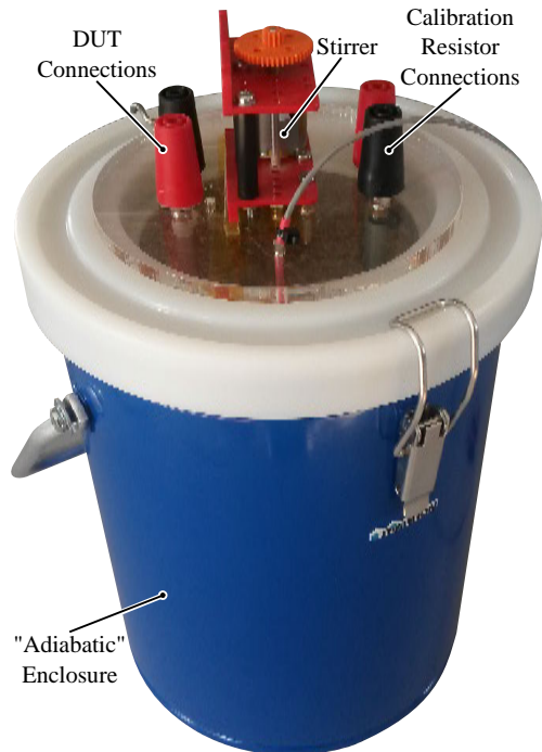
Figure 5.29: Photograph of the calorimeter setup. The DUT size was 7 \times 7 \times 0.45 \text{ cm}^3 . The DUT can have a thickness up to 1 cm. DUT with a cubic shape are limited to 4 \times 4 \times 4 \text{ cm}^3 .
