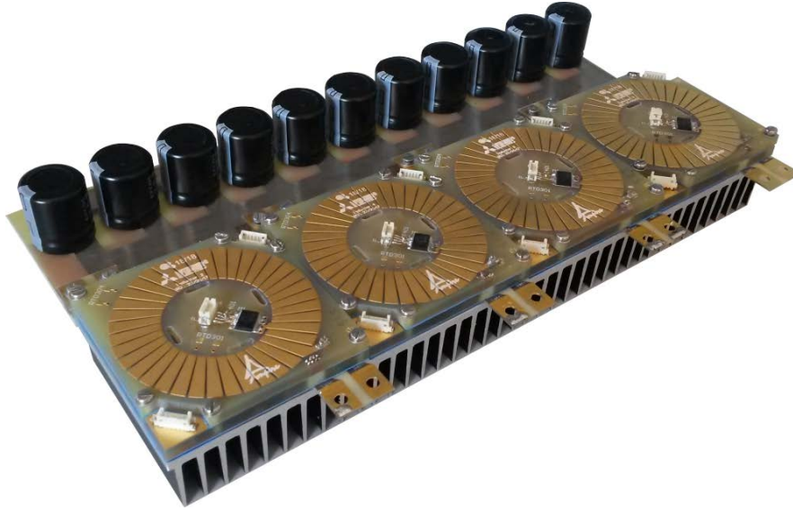
Figure 5.24: Photograph of the PFC with a capacitor bank. The capacitor bank should eventually be replaced by an electronic capacitor to reduce the box volume.
