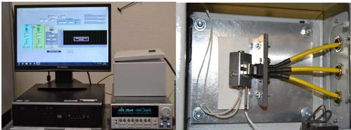
(a) Test-bench used to measure gate-source leakage current. (b) Measurement box of gate-source leakage current.
