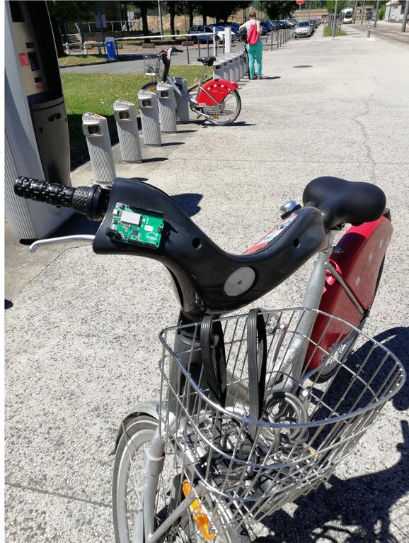
FIGURE A.19: The Things device mounted on Vélo'v bicycle.
