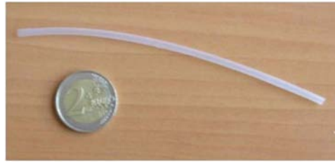
Figure 6: Extruded tube of P(VDF-TrFE-CTFE) with 15% wt
