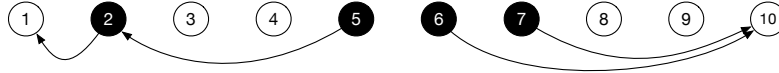
Figure 6.5 – Example with a policy X over n = 10 destinations, with K = 4 destinations (2, 5, 6 and 7) having lost a packet. Arrows indicate recovery requests (SR-NACKs): destination 2 requests recovery from peer 1; destination 5 from peer 2; and destinations 6 and 7 from peer 10; S_X = 3 recovery requests are successful ( i.e. , those from 2, 6 and 7), as peers 1 and 10 have correctly received the original packet; T_X = 2 retransmissions are performed (from 1 and 10).
