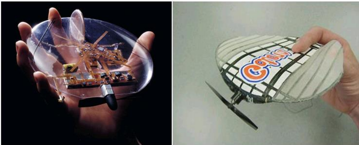
Figure 1.2: Fixed, rigid, and flexible wings, (a) transparent Black Widow by AeroVironment [39], (b) a flexible-wing design developed at the University of Florida [40].
