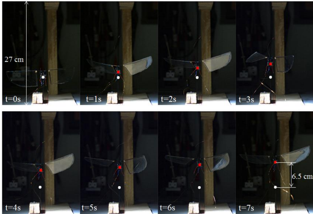
Figure 3.18 : Demonstration of take-off. The white and red dots are the initial and current position of the FWMAV, respectively. After 7 s the vehicle was 6.5 cm above its initial position.
