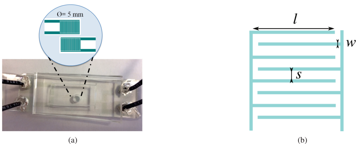
Figure 2.5 – (a) Top view of the ECIS system with bonded PDMS reservoir (5 mm diameter). (b) Interdigitated electrode dimensions: s = 20\ \mu\text{m} , w = 20\ \mu\text{m} and l = 1\ \text{mm} .
