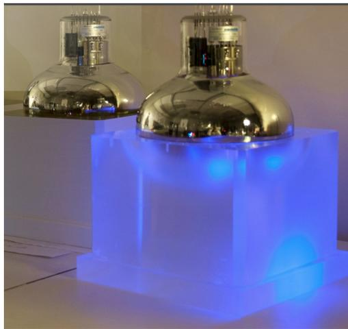
Figure 3.18: Optical module composing the calorimeter before being wrapped into teflon and mylar. The scintillator block is directly coupled to the PMT.
