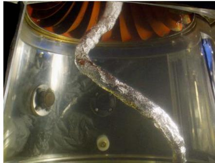
Figure 1.5. Vortex cavitation development downstream a Francis turbine. Source [ICA08]
