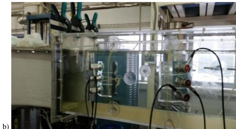
Figure 6.9. Experimental configuration for the asymmetric velocity profile estimation: a) each three sets of “V” paths [E1-R3, E1-E2, E1-R4] and [E2-R1, E2-E1, E2-R2] correspond to emitted signal in the flow direction (the red continuous line), respectively in the opposite direction (the red dotted line); b) The transducers clamp-on open-channel side.
