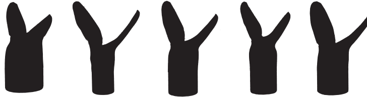
Figure 19: Surfaces exposed to the flow in lateral strike for five models: pc1_{max} , pc1_{min} , mean , pc2_{max} and pc2_{min} (from left to right)
