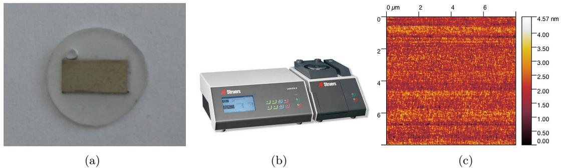
Figure III.3: Picture of pre-strained sample after being embedded with a Mecaprex MA2+ epoxy resin (a). Picture of the apparatus used to electropolish the sample (b). Surface height image in air after electropolishing acquired by scanning probe microscopy (SPM) (c).
