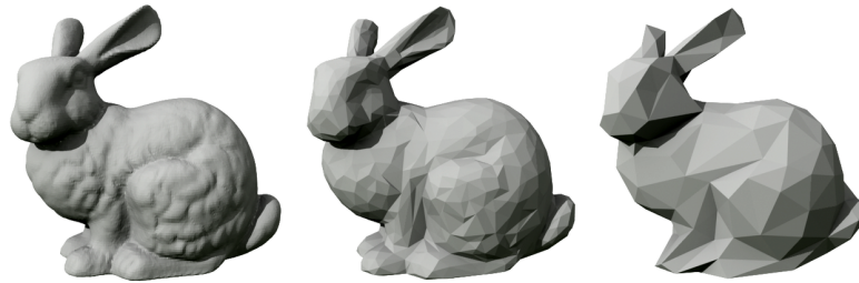
Figure 2.1: Graphical illustration of model reduction [Turk and Levoy, 1994].
