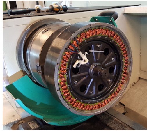
(b) Motor without end shields
