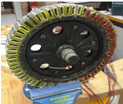
(c) Stator with disassembled windings
