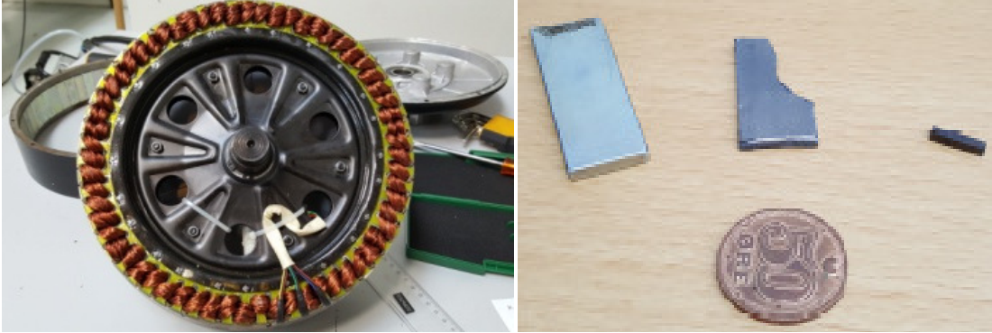
Fig. 4.10 Disassembled machine and permanent magnets
