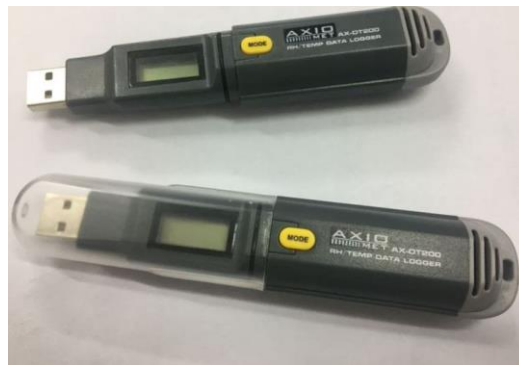
Figure 68: Temperature and relative humidity sensors AXIOMET AX-DT200
