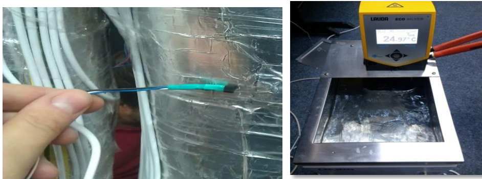
Figure 22: a) TSic T501 sensors used for the measurement and control part of the thermal manikin, b) thermostatic water bath Lauda Eco with immersion thermostat Lauda Eco Silver – The photographs are from the archive of our team during the numerous campaigns of calibrations of the TSic sensors that were also used at another prototype from [215]
