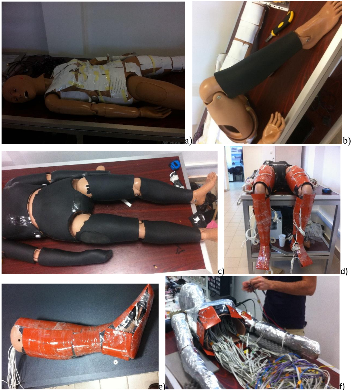
Figure 13: Different stages of making the hardware part of the thermal manikin: a) designing patrons for the heating element disposal, b) and c) designing the heating insulation under the thermal patches, d) inserting the heating elements, e) developing the electrical circuits
