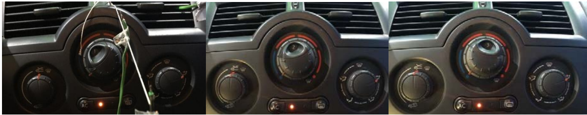
Figure 91: Ventilation system control panel corresponding to the three considered fan velocity steps
