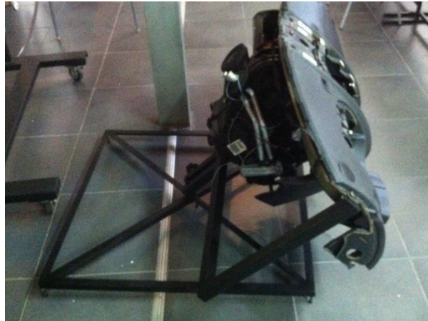
Figure 100: Dashboard and front air ducts mounted on a specially designed structure
