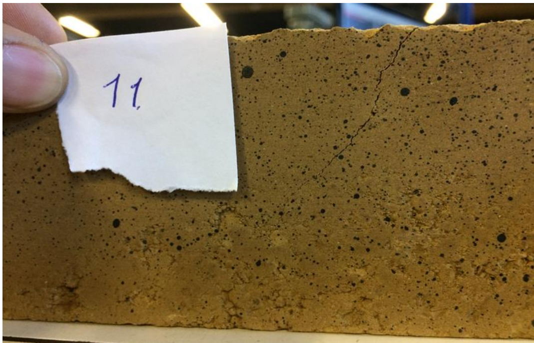
Figure 6-9 An example of speckle pattern
