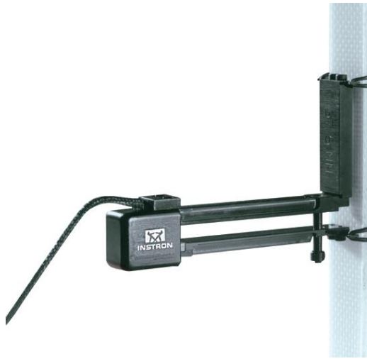
Figure 4-4 INSTRON extensometer 75mm (source: INSTRON website)
