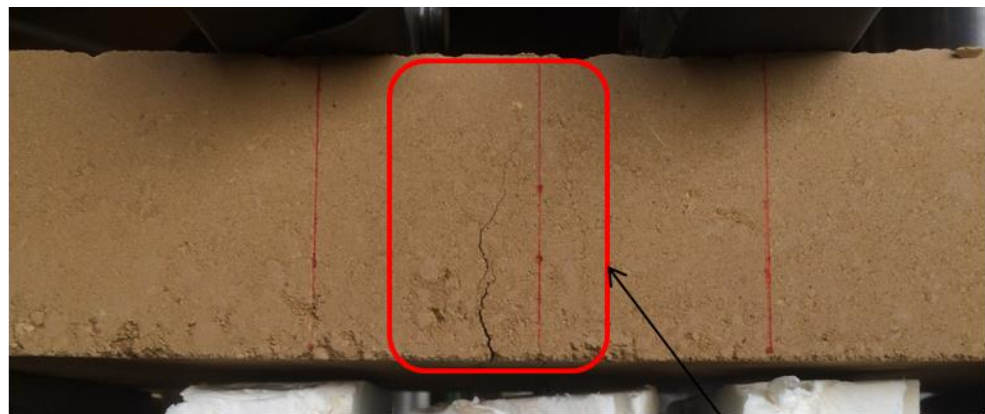
Crack propagation due to tensile stress
