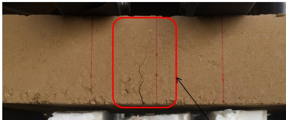
Crack propagation due to tensile stress
