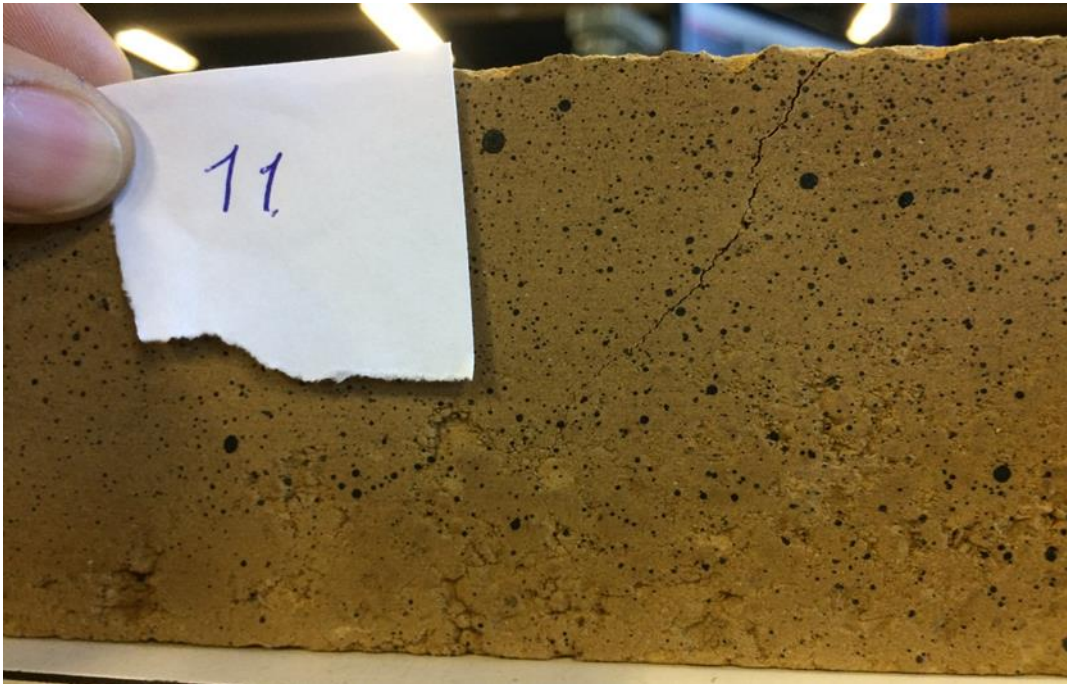
Figure 6-9 An example of speckle pattern
