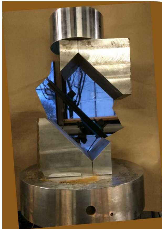
Figure 6-5 Wedge setup to hold specimen in required inclination
