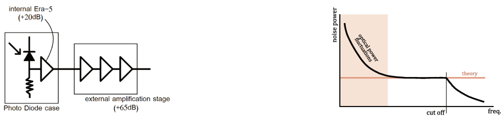
Figure 71: On the left: configuration used for a quick estimation of the thermal noise (electronic noise supposed to be dominated by its thermal contribution) plugged directly onto a wideband FFT. Right: typical expected profile for the photon noise spectrum. The noise diverges for frequency going to zero Hz. For higher frequencies (typically above a few hundreds of MHz) the should be flat till the detector cutoff frequency marking its bandwidth.
