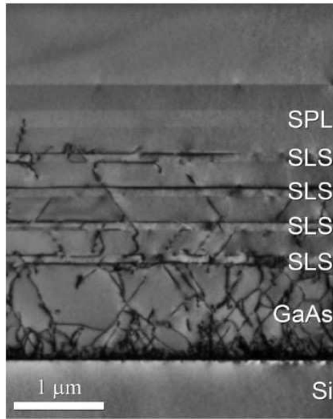
Figure 1.9 Cross-sectional TEM image showing the suppression of threading dislocations through the growth of strained superlattice (SPS) and short period superlattices (SPL). Courtesy of [29]
