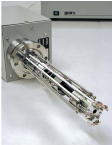
Figure II-20. Hidden analytical quadrupole mass spectrometer 49
