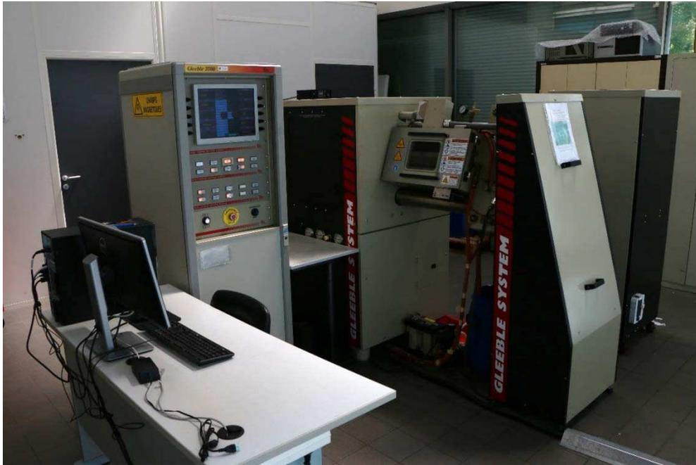
Figure II.11 : Machine Gleeble
