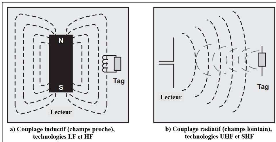
Figure 1-15:Types de couplages RFID [11]
