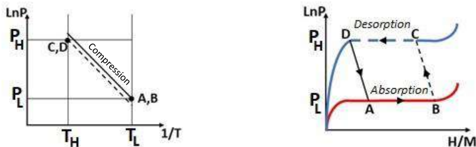
Figure 5.1 Principle of the hydride compressor, van't Hoff plot (left) and ideal P-c-I [1]
