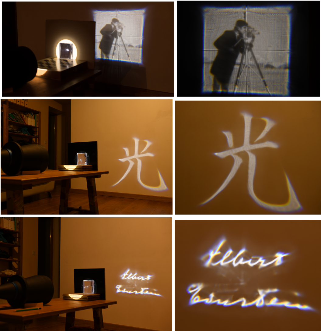
Figure 11 – Fabricated lenses for a collimated light source. From left to right: experimental setup, zoom on the target screen. From top to bottom: CAMERAMAN, HIKARI, EINSTEIN'S SIGNATURE targets. Images are focused on a screen at 2 meters for the first two rows and 1 meter for the last one.
