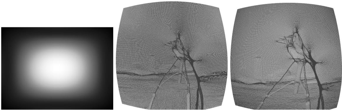
Figure 5 – **Triangulation  $\mathcal{R}_T$  for a non-uniform light source.** *From left to right:* non uniform collimated light source; mesh of the lens for this non-uniform light; mesh of the lens for a uniform light source.
