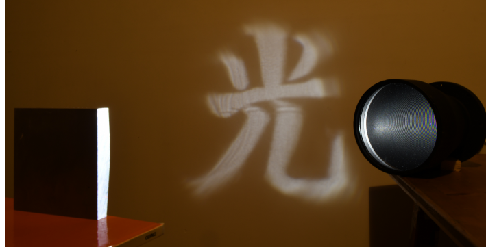
Figure 12 – Fabricated mirror for a collimated light source. HIKARI target. The image is focused on a screen located at 1 meter.
