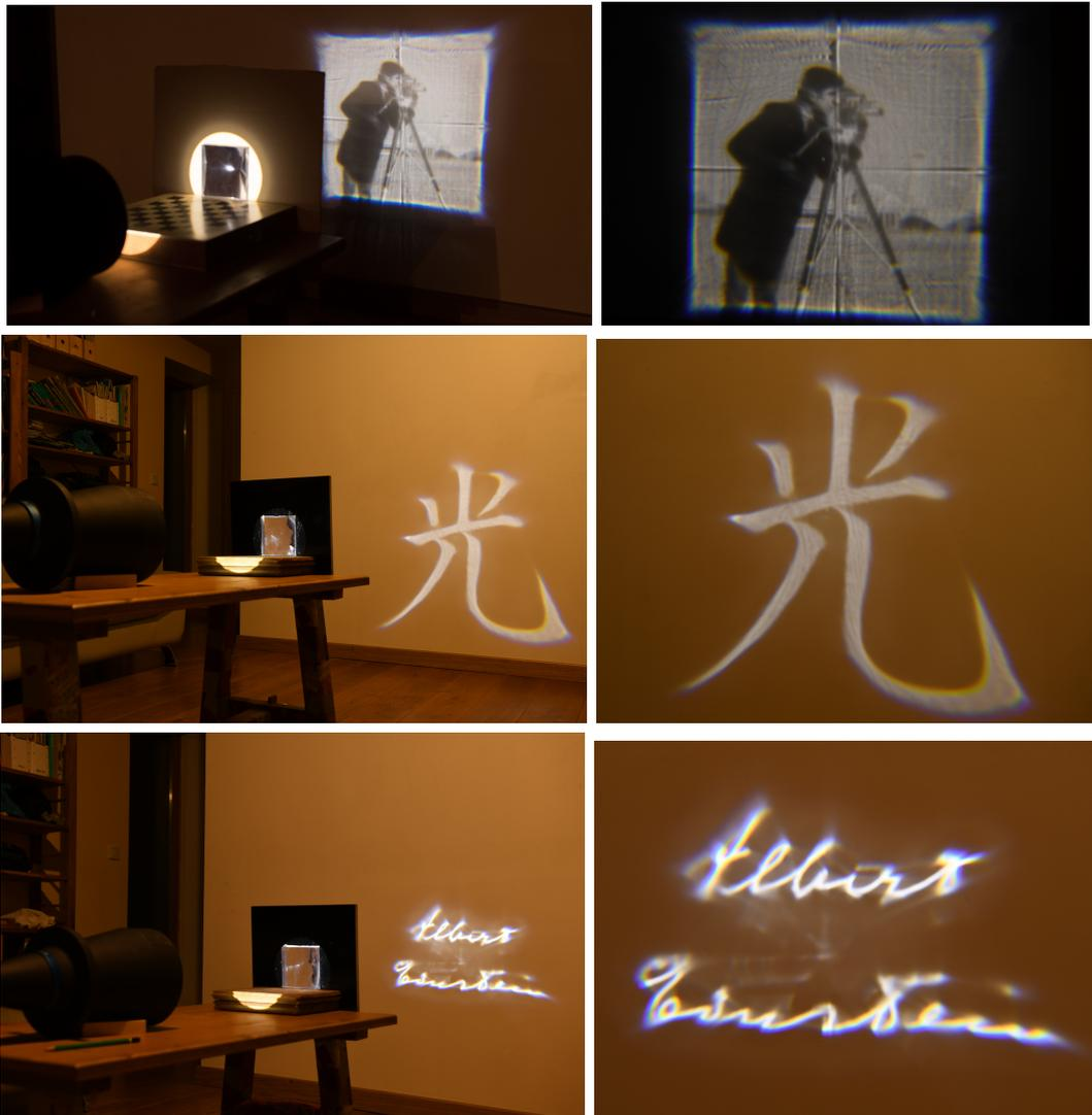
Figure 11 – **Fabricated lenses for a collimated light source.** From left to right: experimental setup, zoom on the target screen. From top to bottom: CAMERAMAN, HIKARI, EINSTEIN'S SIGNATURE targets. Images are focused on a screen at 2 meters for the first two rows and 1 meter for the last one.
