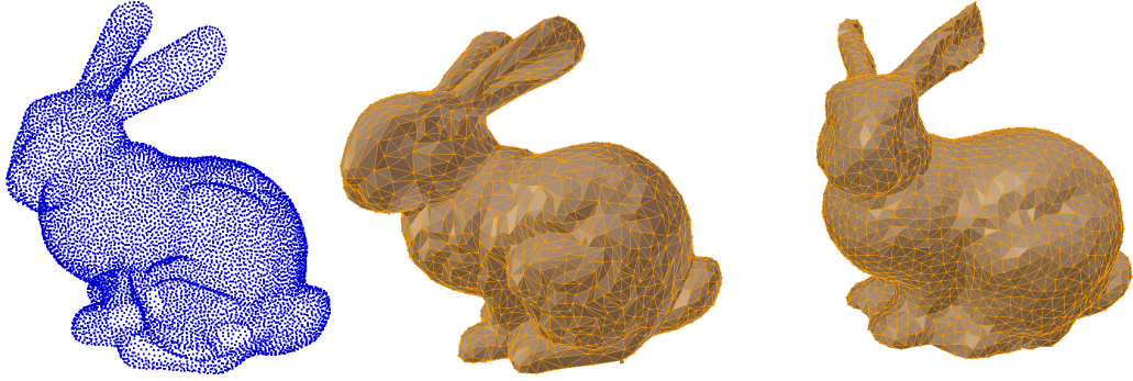
Figure 1 – Examples of applications of optimal transport for source measures supported on triangulated surfaces. Left: optimal quantization of a triangulated surface for a uniform density. Middle and right: remeshing using optimal transport (initial and new mesh).
