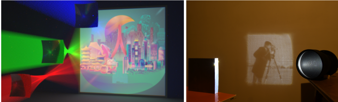
Figure 2 – Examples of simulated and physical results obtained with our method. Left: three lenses that refract the three channels of a color image for three collimated light sources. Right: fabricated mirror that reflects a collimated light source.
