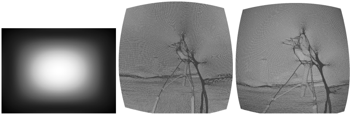
Figure 5 – Triangulation \mathcal{R}_T for a non-uniform light source. From left to right: non uniform collimated light source; mesh of the lens for this non-uniform light; mesh of the lens for a uniform light source.
