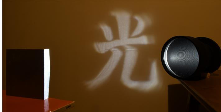
Figure 12 – **Fabricated mirror for a collimated light source.** HIKARI target. The image is focused on a screen located at 1 meter.
